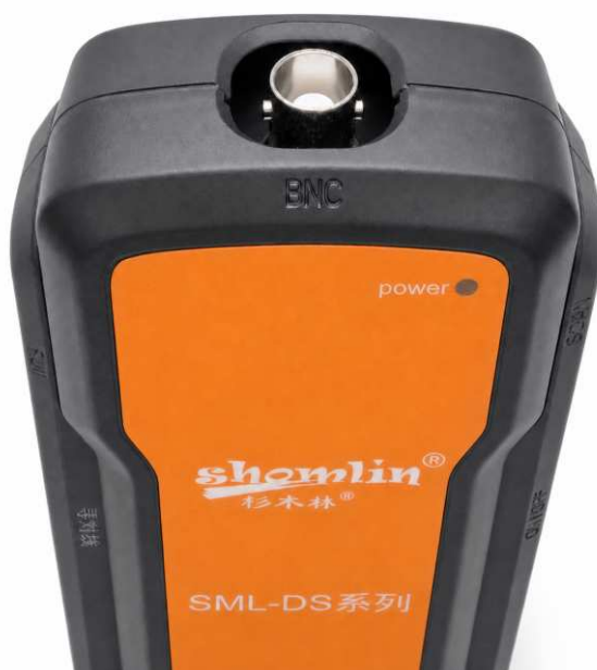
Figure 5-5 Transmitter BNC coaxial tracing port
