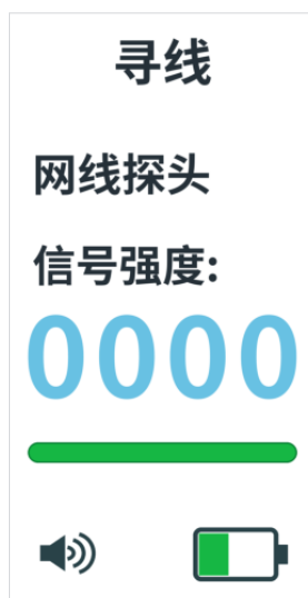
Figure 5-2 Network-cable tracing screen. “网线探头” means “Network Probe,” and “信号强度” means “Signal Strength.”
