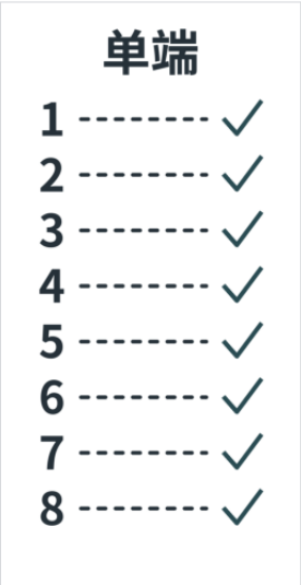
Figure 5-1 Normal RJ45 single-ended test screen. The on-screen label “单端” means “Single-Ended.”
